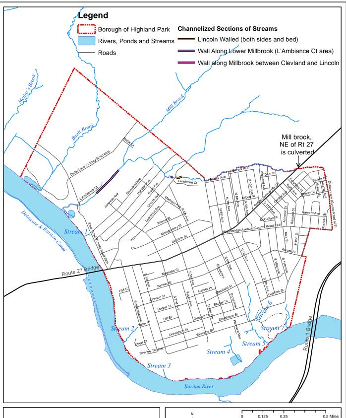
Figure 6d: Streams and Channeled and **Culverted Sections of Streams**
