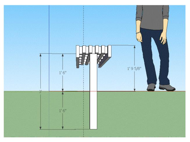
I designed the posts to be 3 feet long, 18" under ground and 18" above ground. This will put the bench seat at 1' 9 5/8" aove ground. This should be comfortable.
