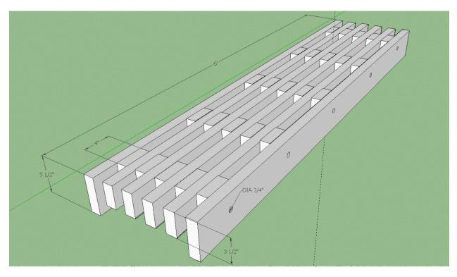
This shows the dimensions for the bench top. the wood pieces will first be glued together with wood glue and then connected with 18" tie rods that will have nylon bolts at each end. the end of the hole will be routed to a \_" diameter to attch the bolts.
